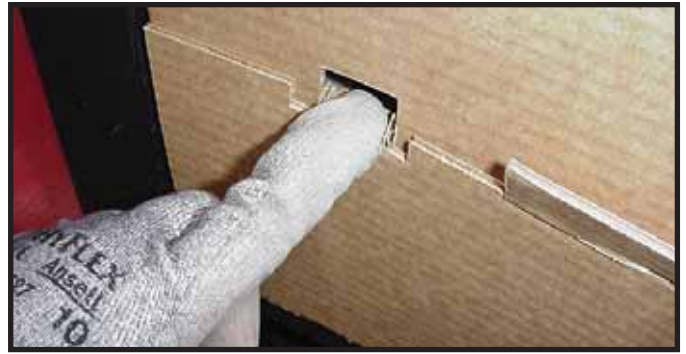
Figure 13.9 Securing Tabs Inside Front of Splatter Guard
